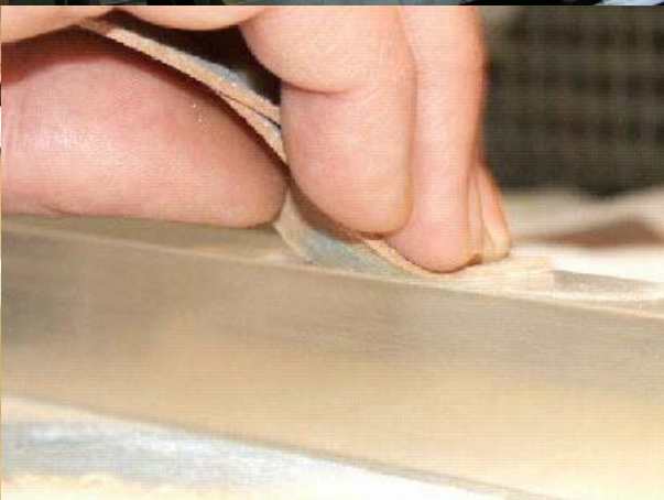
... then a side is scratched ... (tapering)
