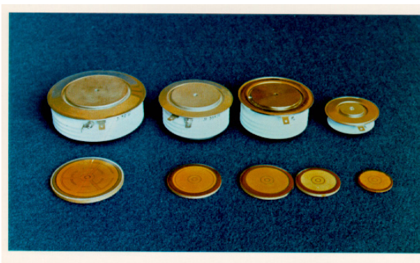
Figure 6. Basic units with their ceramic cases of some power semiconductor devices irradiated with high energy electrons.
